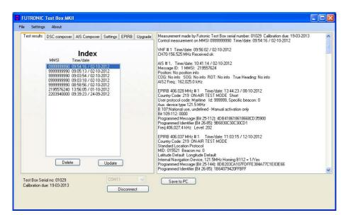
The Futronic MKII comes with free PC software which allows you to view test results and save them to a PC, compose custom-made DSC and AIS messages, generate complete finished EPIRP test reports, personalize test box settings and upgrade the test box with new features.
