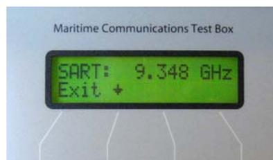
The test box will display the test result in the form of the average frequency of the 12 response sweeps transmitted by the SART along with a figure representing the output power level.
